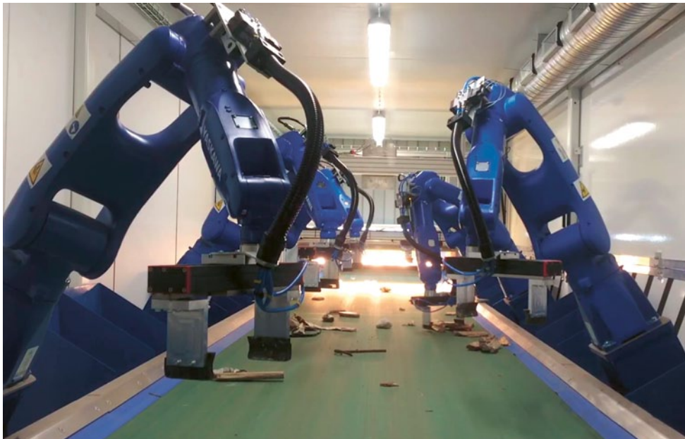
Two robots sorting construction waste. The number of robots is optional.
